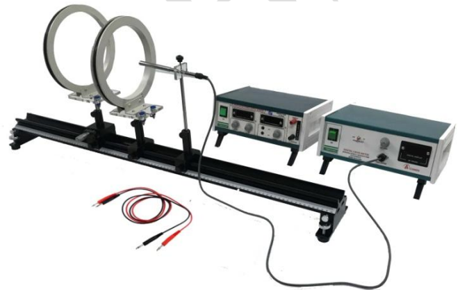
AL-E717 Magnetic Field In Along The Axis Experiment Setup
