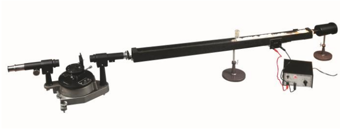
AL-E629 Study Of Absorption Spectrum Of Iodine Vapor.
