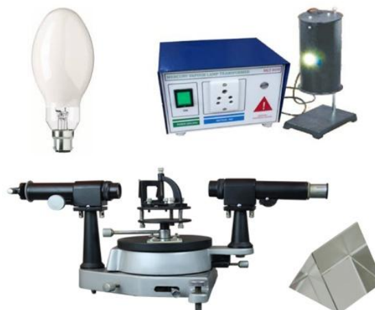
To Determine The Dispersive Power Of The Material Of The Prism For Violet & Yellow Colours Of Mercury Light With The Help Of Spectrometer (Hartmann's Formula)
