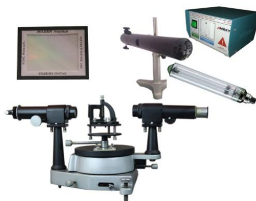
AL-E231 To Find The Wavelength Of Sodium Light Using Diffraction Grating
