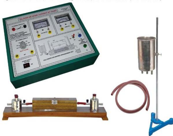
AL-E633A To Determine The Mechanical Equivalent Of Heat By Callender & Barne's Constant Flow Method
