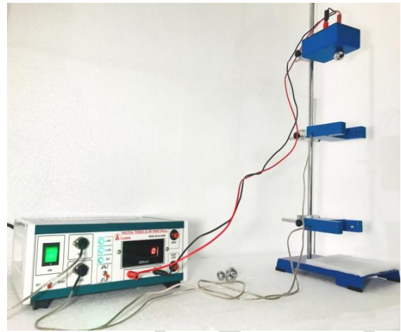
AL-E246 The Measurement Of The Time Of Fall Of A Steel Ball To Determine The Value Of 'G' (G By Free Ball)
