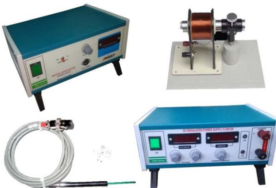
AL-E634 Measurement Of Field Strength B And Its Variation In A Solenoid (Dbdx)
