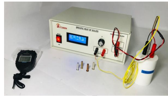
AL-E696 Heat Capacity Of Solid Experiment
