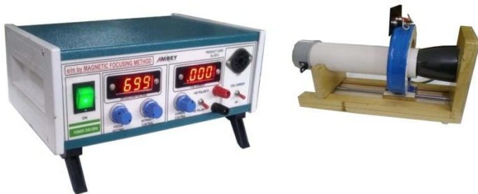
AI-E513 E/ M By Magnetic Focusing Method (Short Solenoid)
