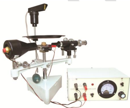
AI-E597 Millikan's Oil Drop Experiment Setup
